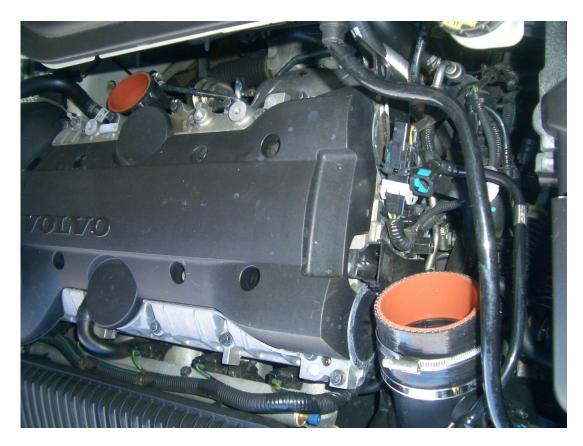
8. Determine if your model requires one or two vacuum line fittings. If only one, leave the cap in place, otherwise, remove cap to allow second connection to be utilized.
