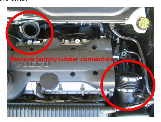
5. The below image shows the engine ready to install the Turbo Intake Pipe.
