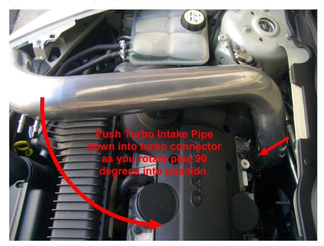
10. Position Turbo Intake Pipe so that it is fully seated into the silicone hose at the Turbo and the silicone connector at the MAF Sensor. Tighten remaining clamps.
