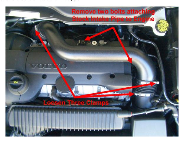
3. Unclip vacuum line from Stock Intake Pipe by depressing tabs and pulling away from pipe. Depending on model, there may be two vacuum lines—remove one or both. Remove Stock Intake Pipe.
