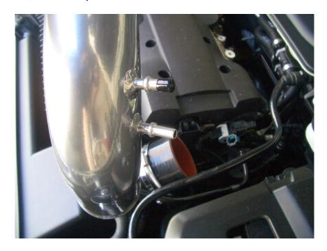
9. Position Turbo Intake Pipe as shown. Press Turbo Intake Pipe down into silicone connector on the turbo as you swing the Turbo Intake Pipe counter-clockwise into position. The Turbo Intake Pipe will not go into position unless this procedure is followed. The Turbo Intake Pipe is a precision fit, and will drop into place.
