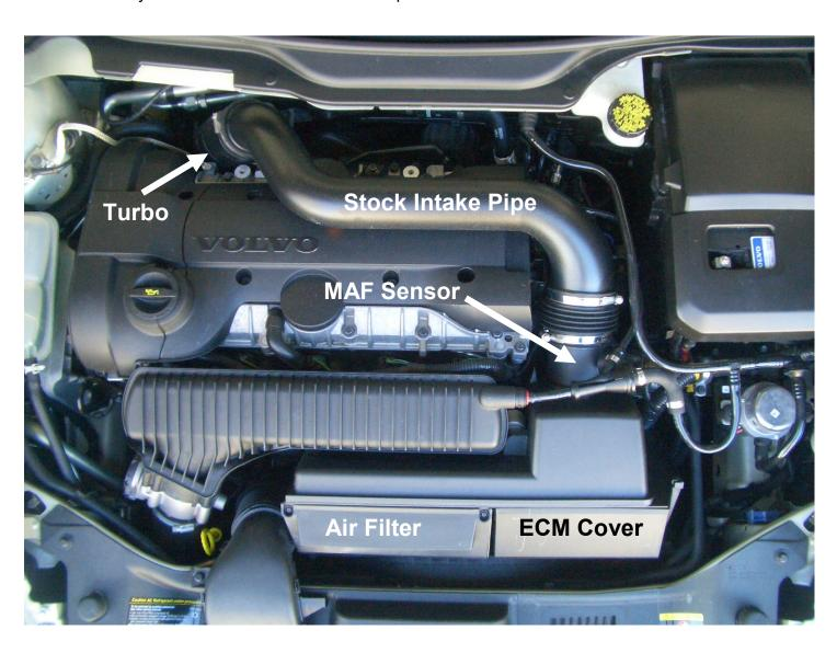
2. Loosen three hose clamps. Remove two bolts attaching plastic pipe to the engine. One of the bolts is under the first bend in the pipe.
