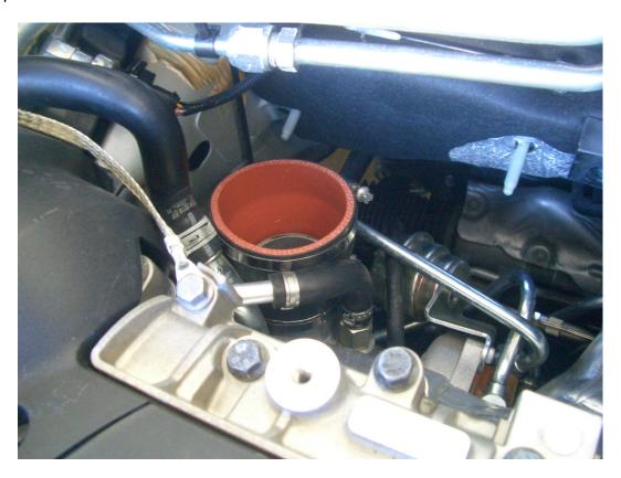
7. Install silicone connector to MAF Sensor using factory clamps. Leave the clamp toward the rear of the vehicle loose.
