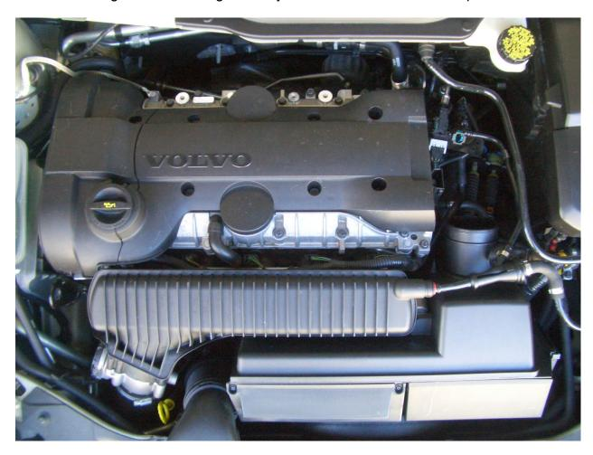
6. Using factory clamp, install silicone reducer hose to turbo. Tighten hose to turbo. Position included clamp on hose in preparation for insertion of Turbo Intake Pipe, but leave upper clamp loose.
