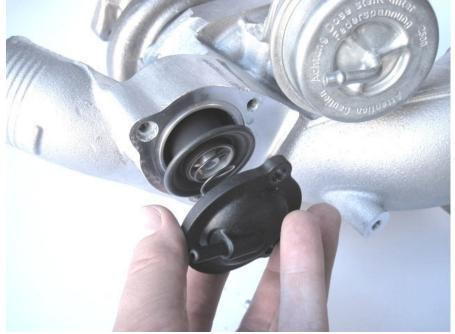
Ensure that all the mounting surface and inside of the compressor housing is clean and free of any dirt or debris. Here you can see the passages that the CBV covers and uncovers in operation.
