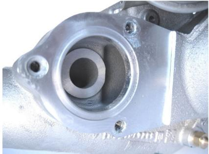
7. Install ELEVATE Turbo Compressor Bypass Valve using included screws and thread locking compound. Make sure both o-rings are in place. IMPORTANT: There is a flat section on the CBV flange. This flat section is to face the turbo compressor inlet. The reason for this is that this is where the opening is for the CBV to redirect boosted air into the turbo inlet.
