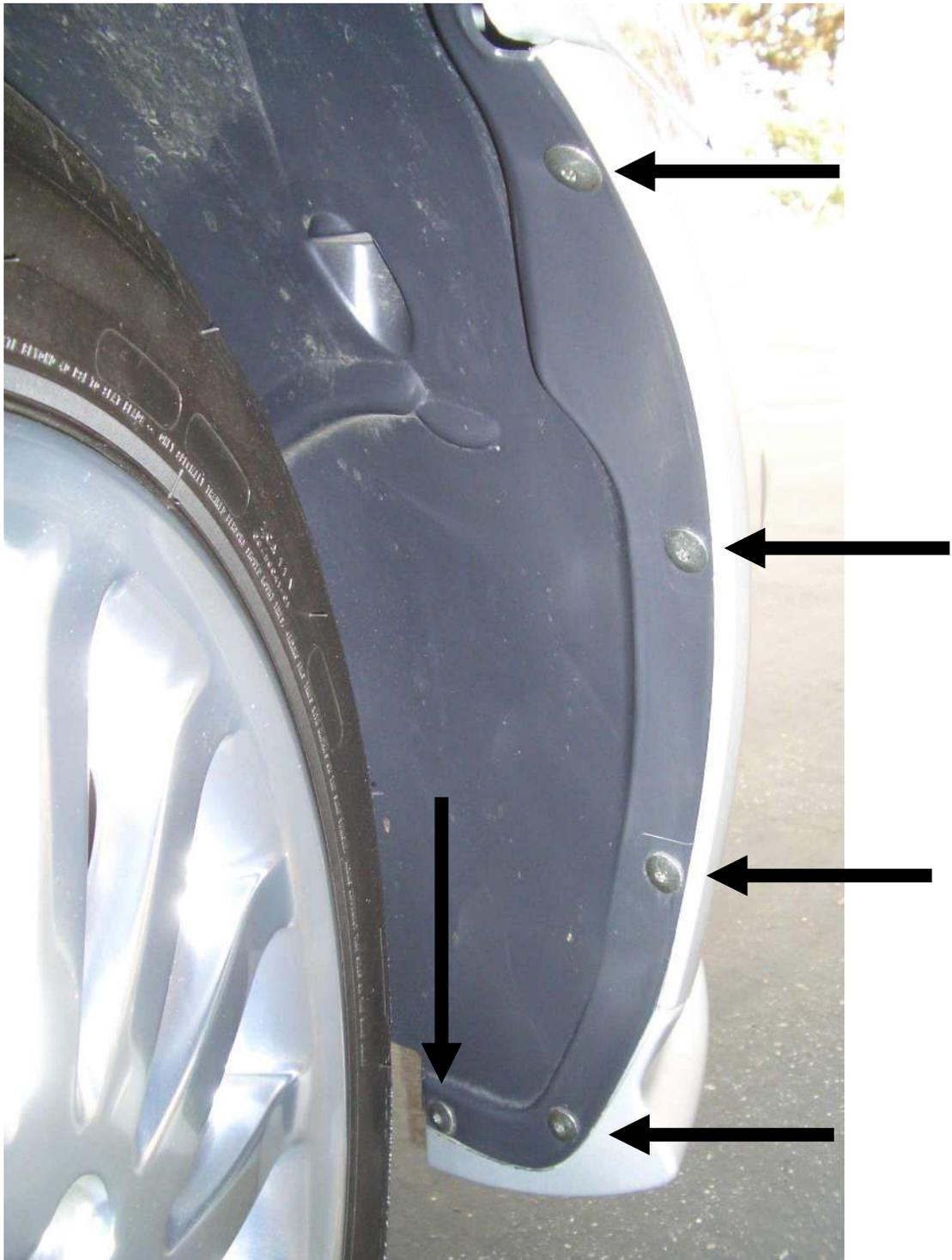
Five T25 Torx screws attach bumper to plastic inner fender.
