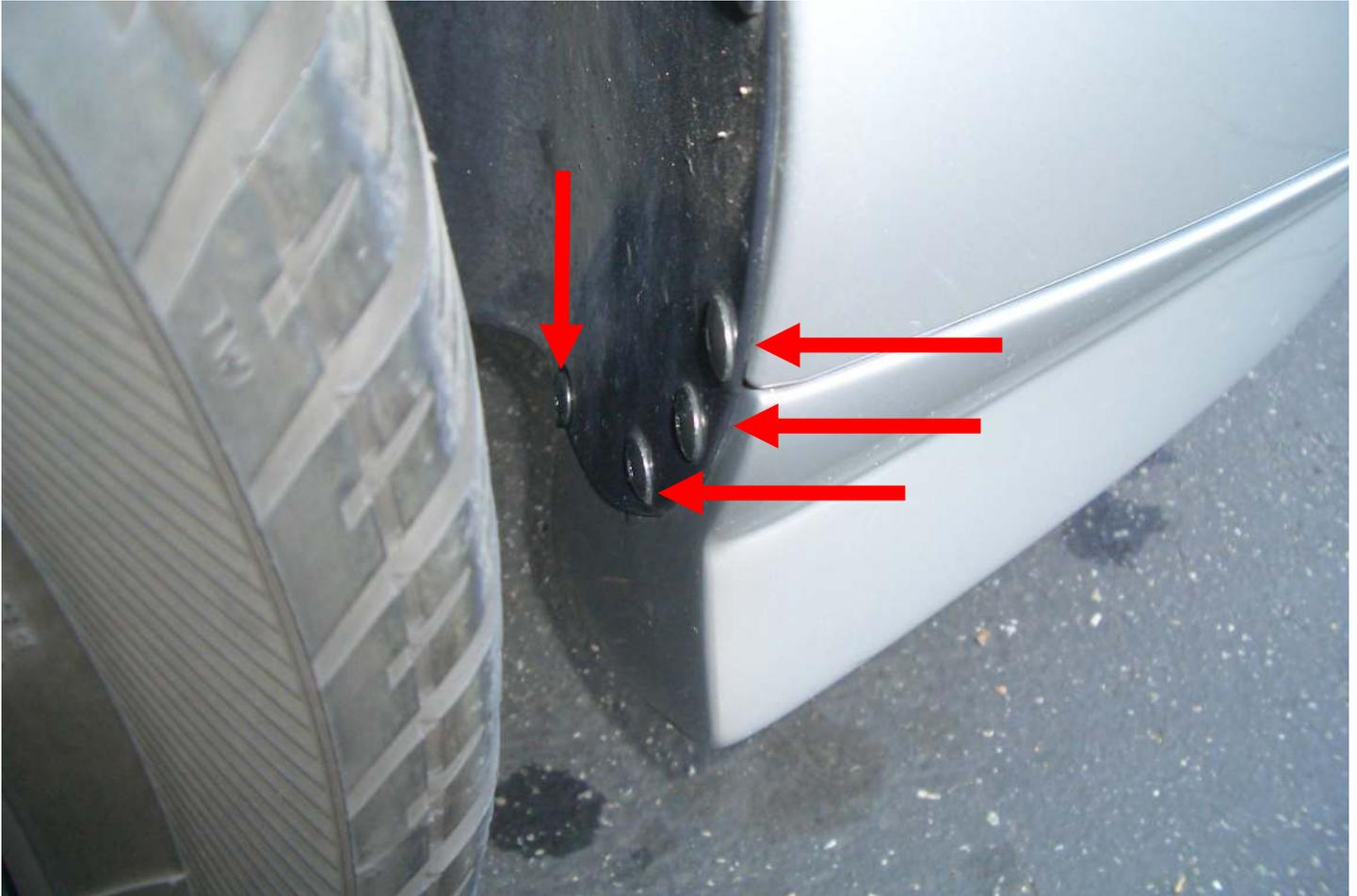
Factory screws secure plastic inner fender to ELEVATE Diffuser
