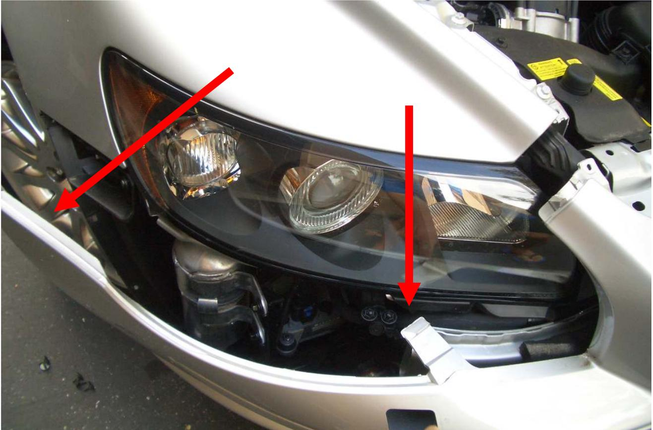
Tabs on top of bumper snap into slot below headlight. Molded section on outer edges of bumper snap into guides that the bottom edge of the front fender.
