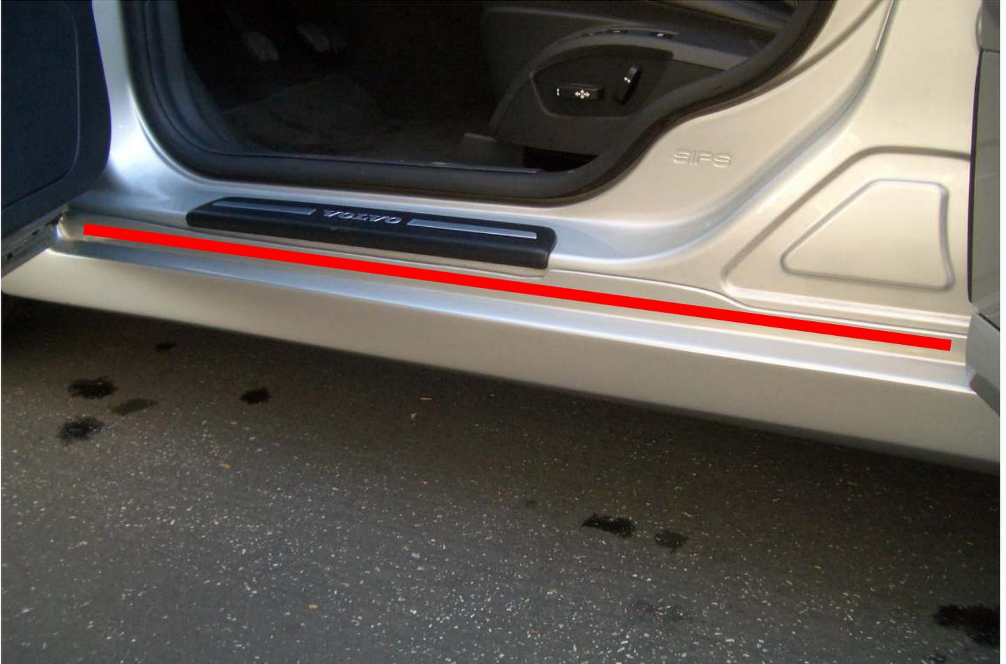
Use double sided tape or rivets to secure upper edge of Side Sill to the lower door sill.
