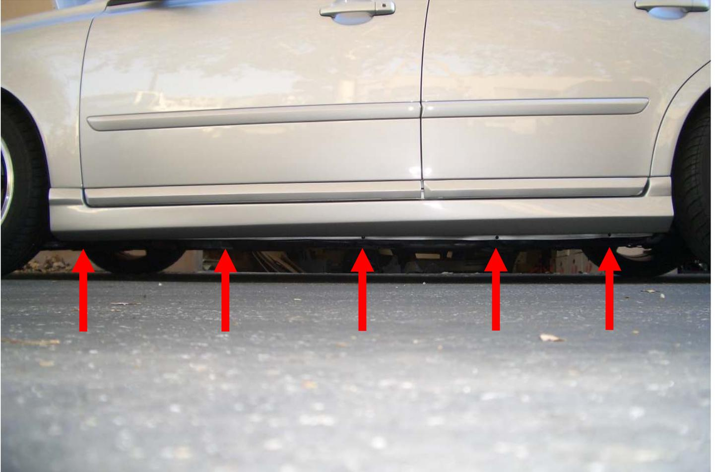
Screws or rivet bottom edge of Side Sill to floor pan rail.
