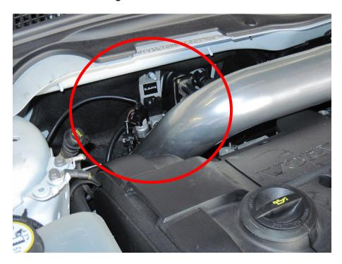
8. Route vacuum hoses and cut to length as detailed below. Use caution when routing hoses as improper routing could cause overboosting or very little boost to be generated. Ports are marked on the valve as "1", "2", "3", with "2" being on the left (when facing valve), "3" in the middle, and "1" on the right.
