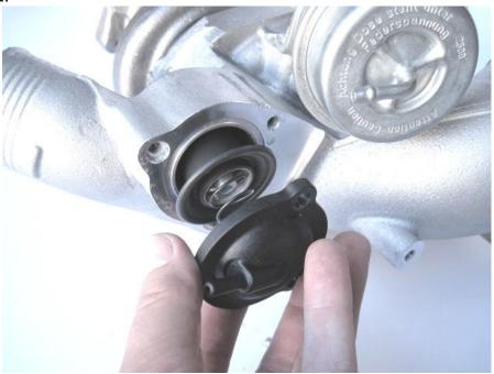
6. Ensure that all the mounting surface and inside of the compressor housing is clean and free of any dirt or debris. Here you can see the passages that the CBV covers and uncovers in operation.
