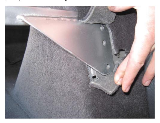
7. Position the seat catch on top of brace bracket and start all four bolts-do not completely tighten. Note that sometimes these bolts need to be run through an M10x1.5 die to clean the threads. The catch brackets have a reference tab and can only be installed one way.
