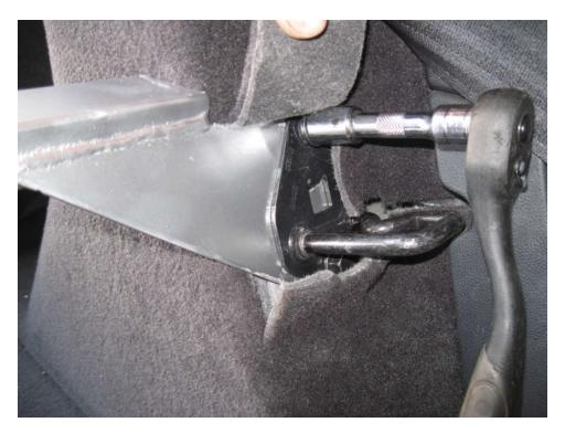
8. Once all four bolts are started and the brace is in the proper position, tighten the bolts securely. Allow the carpet to return to its natural position.
